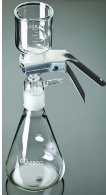
Figure 49. An example of the vacuum filtration unit used to filter biomass samples onto quartz filters for elemental analysis (Growing Labs 2019).
